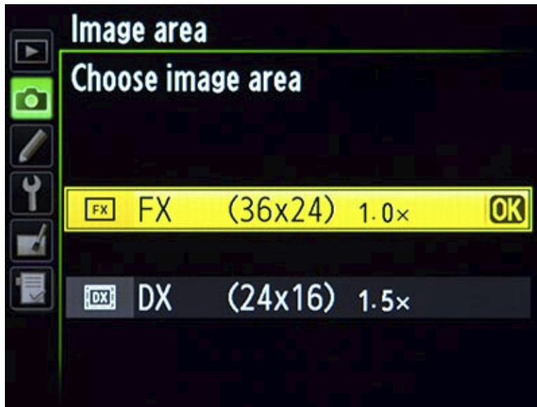
Figure 33 - Image Area option - choose to have your full size FX format sensor capture images full size (FX) or cropped (DX) as if using an APS-C sensor sized camera.
