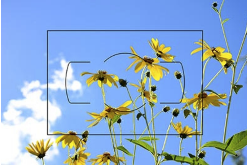
Figure 31 - Simulated D610 Viewfinder view, showing the full size FX image area and the approximate size of the cropped DX image indicated by the inner black line surrounding the AF brackets. Note that the DX image size aligns approximately with the Viewfinder Grid Display lines which can be turned on with Custom Setting d2.
